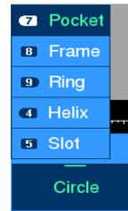
Additional milling functions are available by pressing the **Program Steps** soft key. The soft keys change, displaying several Milling function soft keys. Each soft key when selected will have a popup menu for further selection to refine the type of milling operation to be entered. For example, the **Circle** soft key will display choices for the type of circle to be milled; a Pocket, Frame, Ring, or a Helix.
