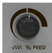
Adjustment of the feed rate with the potentiometer can be done at any time, even while the table or quill is moving.
